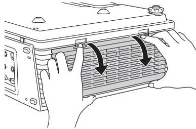
4. Remove the air filter by pulling the center of air filter straight out.
