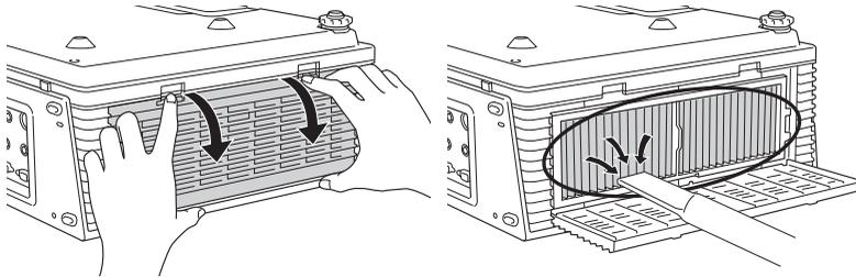
3. When you have finished cleaning the air filter, close the cover and reset the timer as described on page 92.
