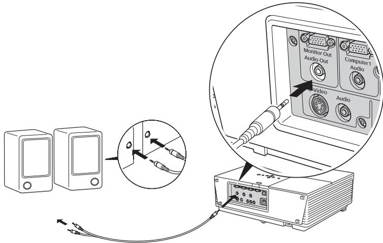
3. Connect the other end(s) of the cable to your speaker system. You may need to use an adapter to make the connection.
