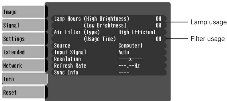
The lamp typically lasts from 2500 to 3000 hours, depending on the selected Brightness Control setting (see page 57). If the number shown is close to that, make sure you have a spare lamp handy. If you've installed a new lamp, be sure to reset the lamp timer (see page 95).
