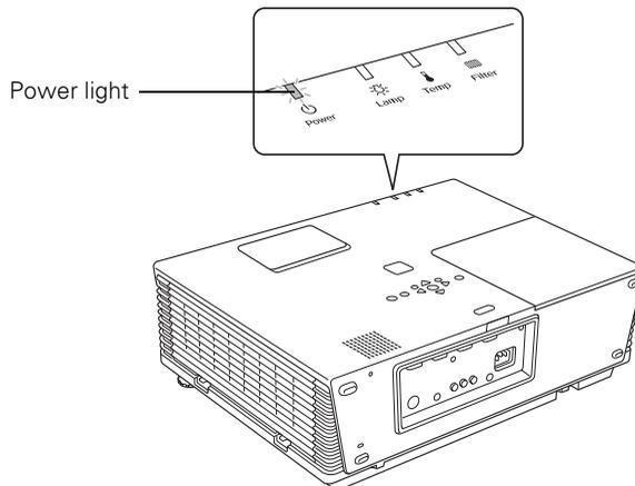
3. Press the orange
