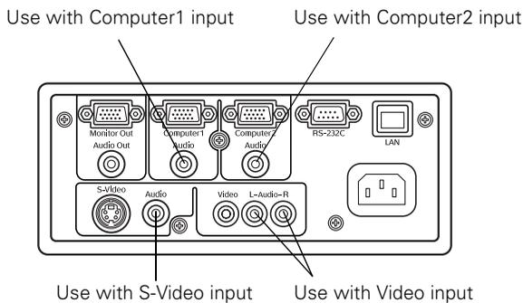
3. Connect the other end of the cable to the audio-output connector on your computer or video equipment.
