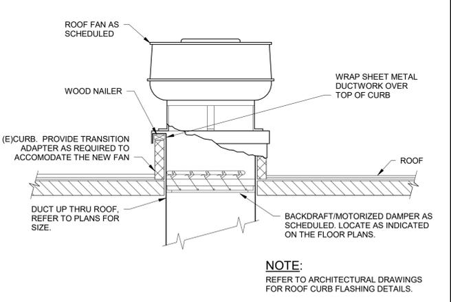
A8 DETAIL - ROOF MOUNTED EXHAUSTER
