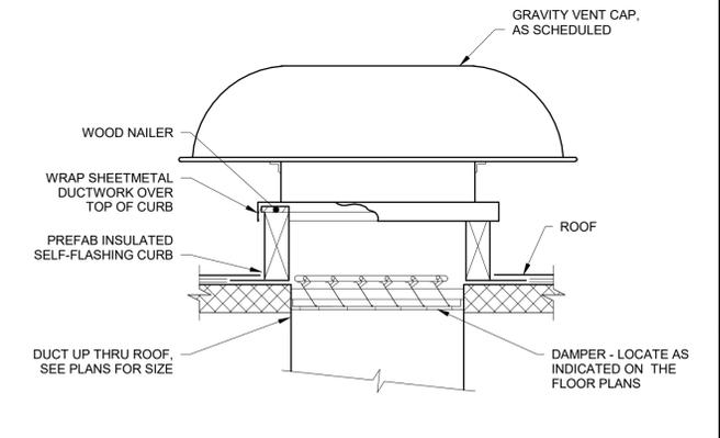
C8 DETAIL - ROOFTOP GRAVITY INTAKE/RELIEF
