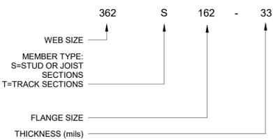
THE LAST TWO NUMBERS INDICATE THE STEEL THICKNESS
