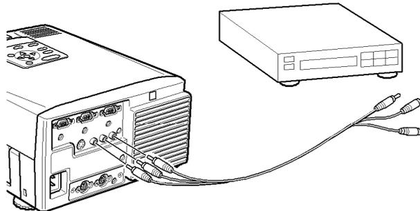
4. Connect the other plugs on the audio/visual cable to the Audio In jacks of the projector: insert the white plug into the L Audio In jack and the red plug into the R Audio In jack. Connect the plug at the other end of the audio/visual cable to the audio output jacks of the video source.
