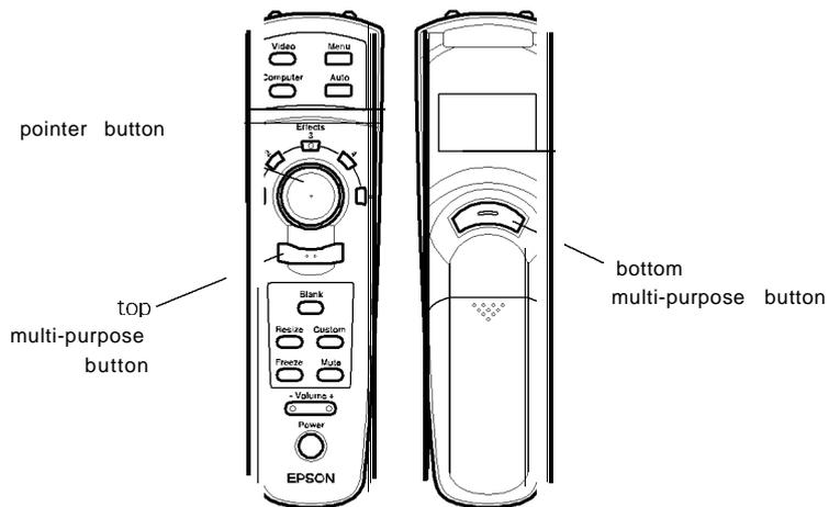
The remote control uses a line-of-sight infrared signal. To use the remote control, point it towards one of the remote control receivers located at the front and back of the projector.
