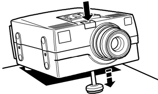
1. Stand behind the projector and support the front of it while you press the purple button above the lens. This unlocks the foot so it can move up and down freely. **DO** not let the projector drop.
