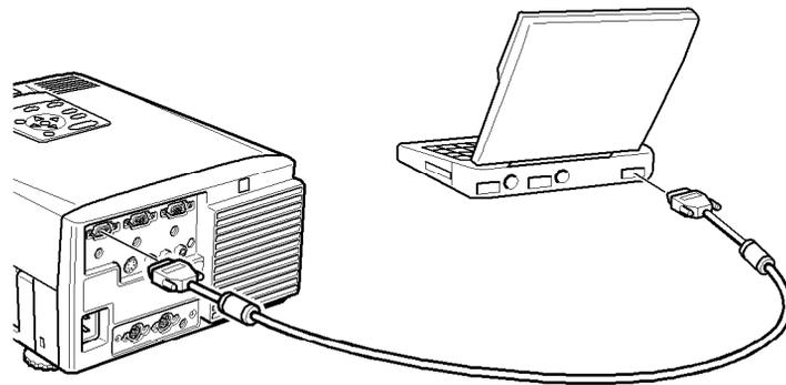
**Note:** Laptop configurations vary. See your computer manual for the location of the ports needed to connect your PowerLite 5000 projector.
