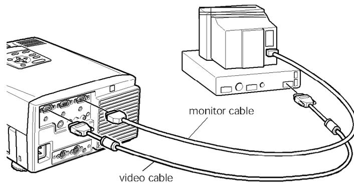
**Note:** Computer configurations vary. See your computer manual for the location of the ports needed to connect your PowerLite 5000 projector.
