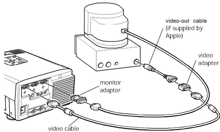
**Note: Macintosh computer configurations vary. See your computer manual for the location of the ports needed to connect your PowerLite 5000 projector.**
