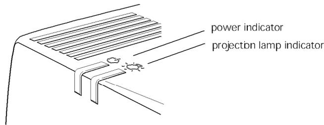
When the projector has cooled off, flashing stops and the power indicator changes to orange.
