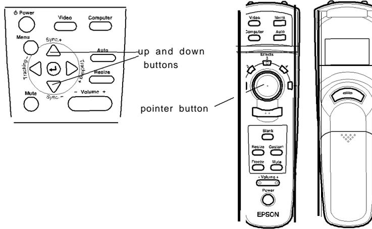
3. Press either the Enter button (control panel) or the top or bottom multi-purpose button (remote) to display a submenu.
