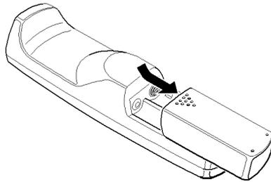
6. Insert the two AA batteries included with the projector. Make sure the polarity of the batteries is correct.
