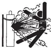
**CYLINDER HANDLING -- Cylinders, if mishandled, can rupture and violently release gas. Sudden rupture of cylinder, valve, or relief device can injure or kill. Therefore:**
