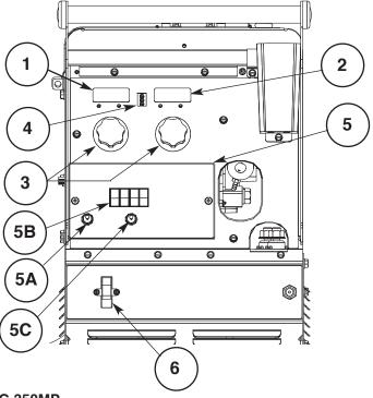
2. VOLT / TRIM METER - This meter displays either the voltage or trim value depending on the status of the machine. Located below the display is the text "Volts" and "Trim." An LED light is illuminated to the left of one of these in order to indicate the units of the value displayed in the meter.
