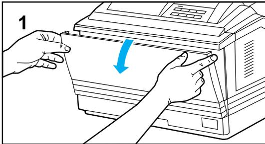
**1** Open the MP tray by grasping the door on the front of the printer, at the pattern of raised dots on each side. Pull the tray down gently until it stops.
