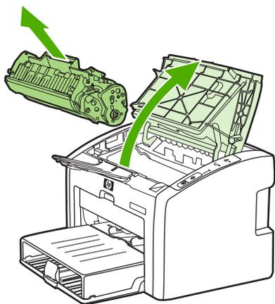
3. With a dry, lint-free cloth, wipe any residue from the media path area and the print cartridge cavity.
