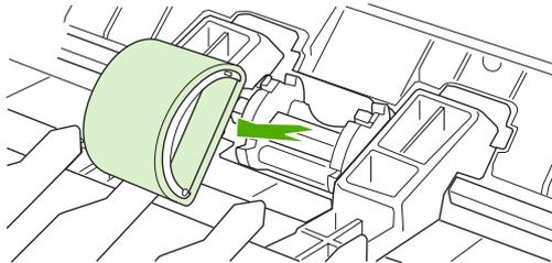
6. Position the new pickup roller in the slot. The circular and rectangular slots on each side will prevent you from installing the roller incorrectly.
