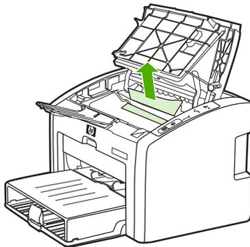
3. When you have removed the jammed media, replace the print cartridge, and close the print cartridge door.
