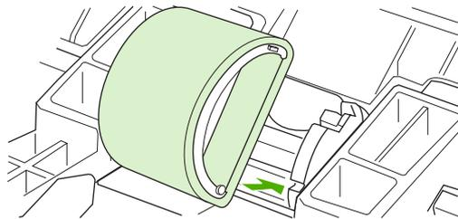
7. Rotate the top of the new pickup roller away from you until both sides snap into place.
