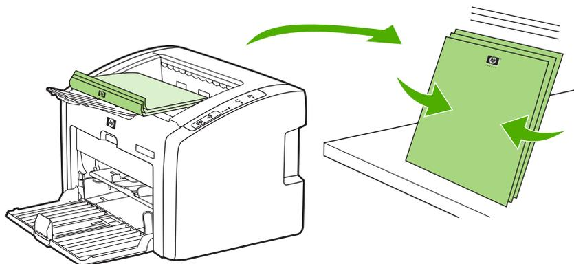
5. Place the stack back in the input tray. Side one should be facing down with the bottom edge feeding into the printer first. Replace the media input tray cover.
