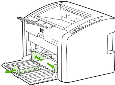
3. Place the envelopes with the side to be printed facing up and the top edge along the left media guide. Stack up to 15 envelopes.
