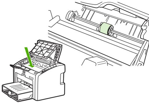
4. Release the small, white tabs on either side of the pickup roller, and rotate the pickup roller toward the front.
