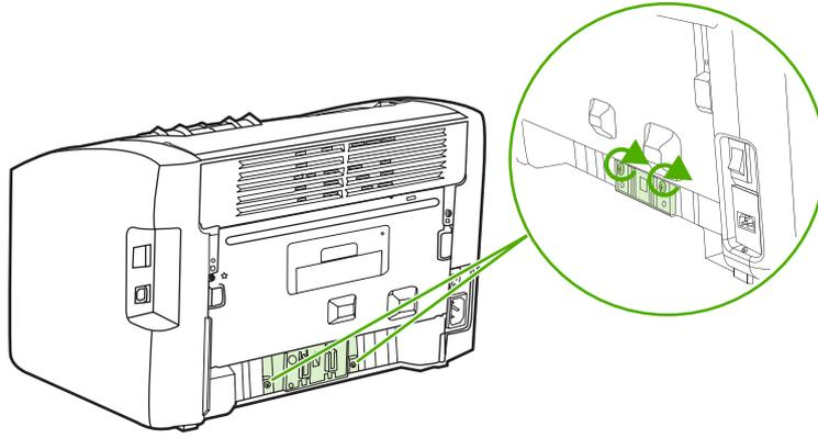
5. Plug the printer into the power outlet, and turn on the printer.
