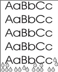
A diagram showing five lines of the text 'AaBbCc'. At the bottom edge of the page, there are several small water droplets. | <p><b>NOTE</b></p> <p>Moisture in the printer is condensing on the fuser assembly and dropping onto the media. In excessively hot and humid areas, media retains moisture. Water droplets do not damage the printer.</p> <ul style="list-style-type: none"><li>• Use different media.</li><li>• Store media in an airtight container to minimize absorption of moisture.</li></ul> |
