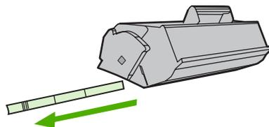
4. Insert the new print cartridge in the printer, making sure that the print cartridge is in position. Close the print cartridge door.
