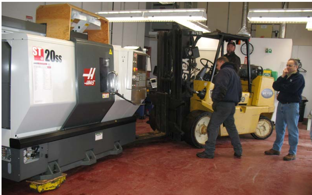
Dean Duplessis (far right), lead instructor of Northern Maine Community College’s precision metals manufacturing program, looks on as a new state-of-the-art Haas automation lathe was delivered and installed in the college’s CNC lab recently. The $110,000 piece of equipment was provided as the result of a school entrustment agreement with Haas Automation, Inc.
