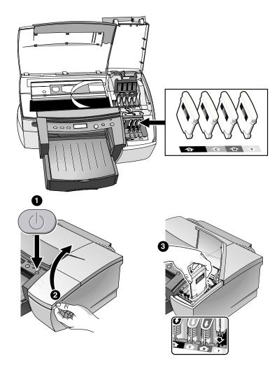
**D** Press firmly on the cartridges to ensure proper contact.
