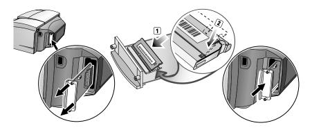
If your printer has the HP PCL 5C/Postscript 3 emulation card installed, you may install up to 128 MB of additional memory which is available for purchase as an accessory (part number C2388A).
