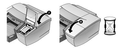
**K** Wait while the printer initializes the printheads. This can take up to 8 minutes. When initialization is complete, an alignment page prints. If no alignment page prints, check to make sure there is media in the trays.
