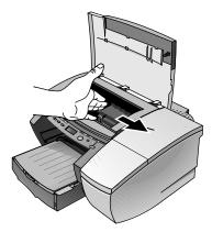
4 Free any wrinkled paper and pull the sheet of paper towards you through the front of the printer.
