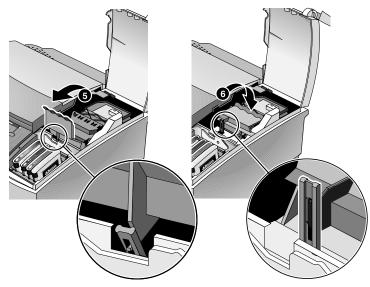
push the latch towards the back of the printer. You might have to apply some pressure to close the printhead access latch.
