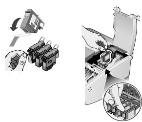
G Insert each printhead into its color-coded socket.
