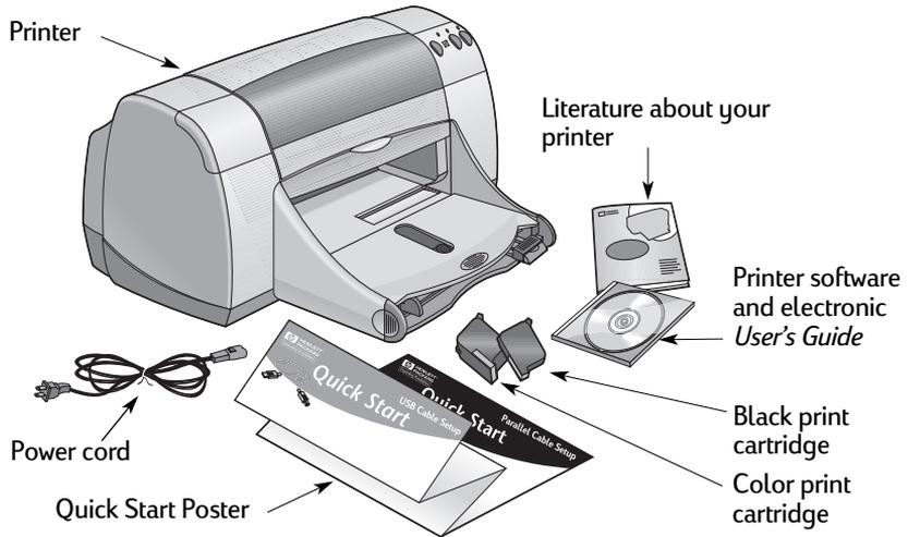
**Note:** You'll need to buy a printer cable, such as the HP IEEE 1284-Compliant Parallel Interface Cable (bidirectional). If you are using Windows 98 and want to use a USB connection, purchase an HP USB-Compliant cable (see "Ordering Information" on page A-7 in the Electronic Appendix). Access the Electronic Appendix from the HP DeskJet Toolbox (see page 8).
