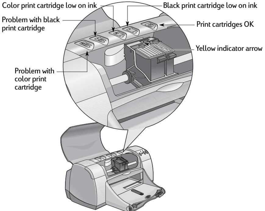
When the Print Cartridge Status Light flashes, open the printer's top cover and follow the instructions below. For more information on replacing print cartridges see page 27.
