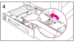
Load up to 500 sheets of 20 lb  $(75 \text{ g/m}^2)$ bond paper in trays 2 and 3.
