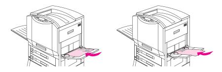
The duplexer prints the second side of the paper first, so paper such as letterhead and preprinted paper needs to be oriented as shown.
