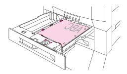
Place the media into the input tray with the side to be printed on face down (see figure 10) for single-sided printing.
