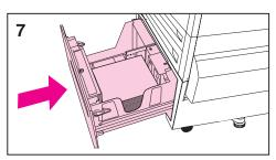
5 Load up to 2,000 sheets of 20 lb (75 g/m²) bond paper into the input tray. For information on loading different types of media, see "Orienting Media for All Other Trays" later in this chapter.
