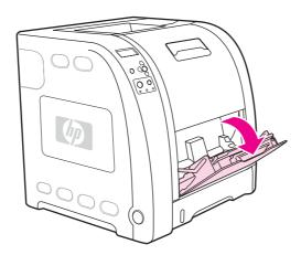
2. Slide out the tray extender and, if necessary, open the additional tray extender.
