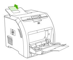
3. Slide out the tray extender and, if necessary, open the additional tray extender.
