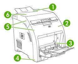
Figure 8-1 Jam locations (printer shown without optional tray 3)
