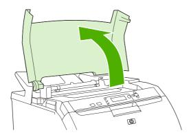
2. If the jammed sheet is visible, remove it and then close the top cover.
