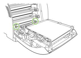
**4.** Press the tabs, and then lift the registration plate. Remove any jammed media, and then return the registration plate to its closed position.
