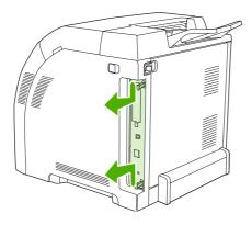
3. Place the formatter board on a clean, flat, grounded surface.
