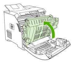
4. Remove any jammed sheets from under the transfer unit.
