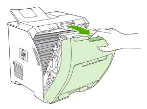
3. Rotate the transfer unit up and away from the front door.
