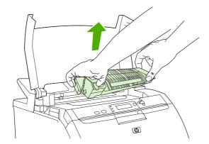
**5.** On the fuser, lift the shutter door.
