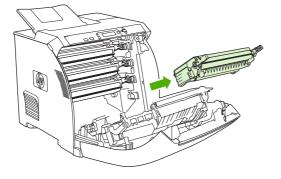
3. Remove the new print cartridge from the bag. Place the used print cartridge in the bag for recycling.
