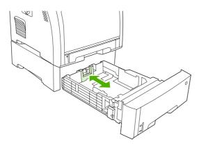
4. Move the side width guides until the arrow on the right width guide points to the size that you are loading.
