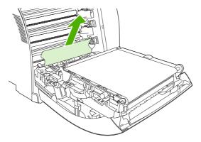
3. Locate the green registration-plate tabs that are below the bottom print cartridge.
