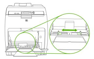
4. Load as many as 10 envelopes in the center of tray 1 with the side to be printed on facing down, with the stamp area farthest from the printer, and the short edge toward the printer. Slide the envelopes into the printer as far as they will go without forcing them.
