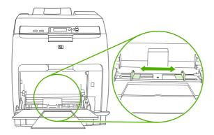
5. Place print media into the tray with the side to be printed down, and the top, short edge in first.
