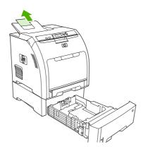
3. Adjust the length guide until the arrow points to the size that you are loading.
