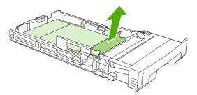
5. If the sheet is not visible, check inside the printer at the top of the tray opening. Remove any jammed media.
