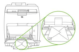
5. Adjust the guides to touch the envelope stack without bending the envelopes. Make sure that the envelopes fit under the tabs on the guides.
