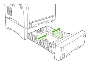
5. Load the media into the tray. If this is special paper, such as letterhead, load it face-up with the top edge toward the front of the tray.
